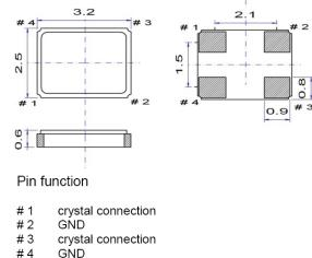
Pad #2 & #4 connected with the metal cap
