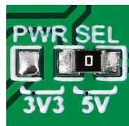
The board features a PWR SEL jumper which is used to determine whether 5V or 3.3V power supply is used.
